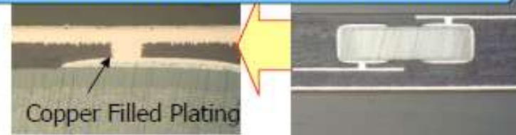
Cross section of PWB with embedded Components
